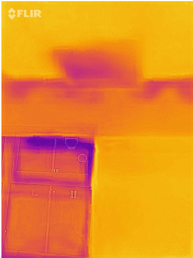
Bedroom ceiling showing missing loft insulation
