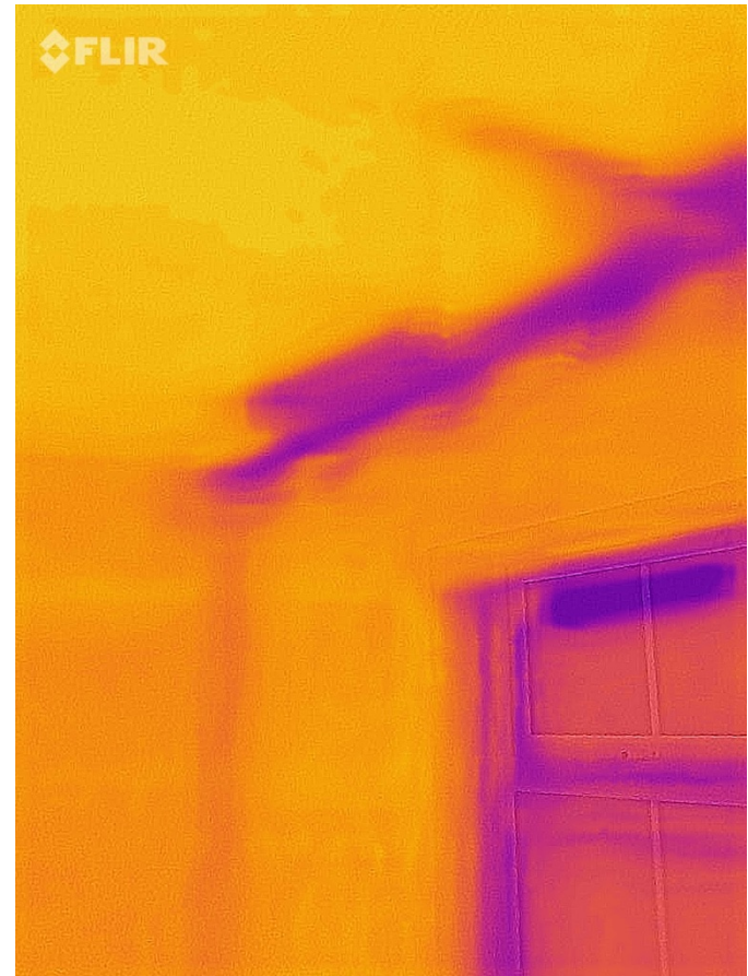
Bedroom ceiling showing missing loft insulation
