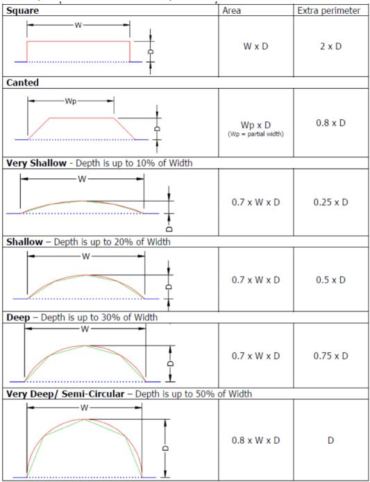
To calculate the total perimeter measure the whole length of wall, including bay, and add the Extra Perimeter to the length.
