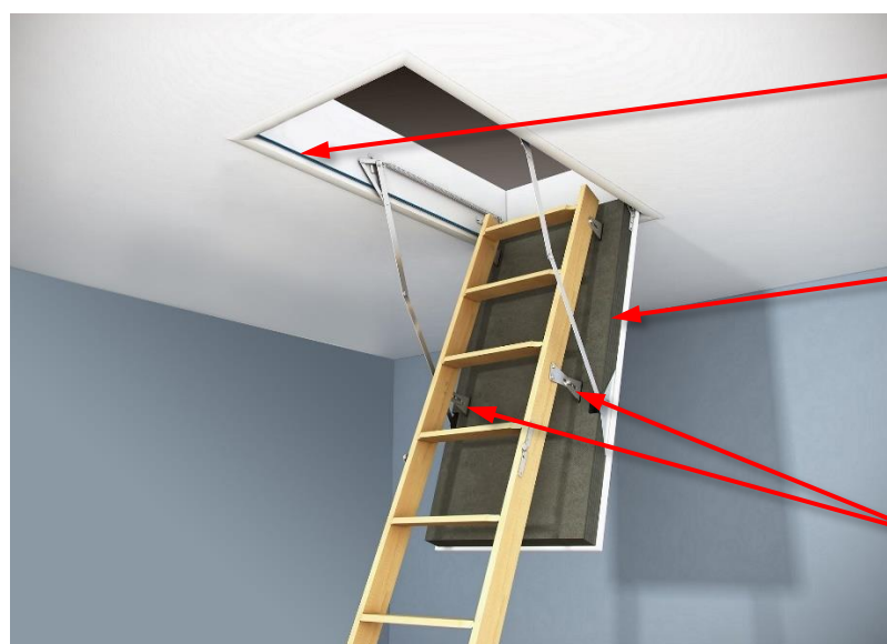
Figure 4 Hatch with fixed ladder with retrofit insulation and draught proofing
