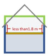
RR Type 2 has an accessible vertical continuation of the external wall of the storey below which is **less than 1.8 m** for at least 50% of the common wall (excluding gable ends or party walls).
